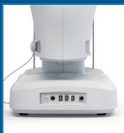
Connectors on the back include 3 USB ports and 1 Ethernet port.
